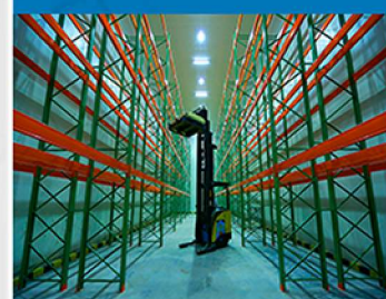
Double Deep Pallet Racking
