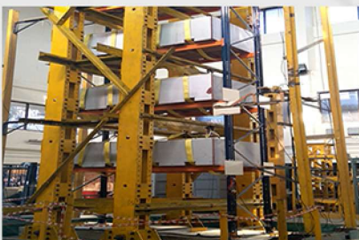
Tested seismic racking
