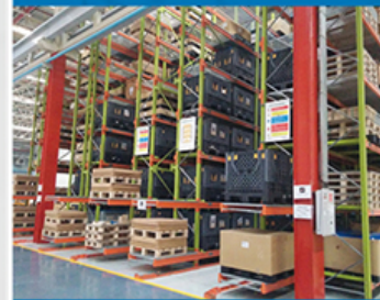
Very Narrow Aisle Pallet Racking System
