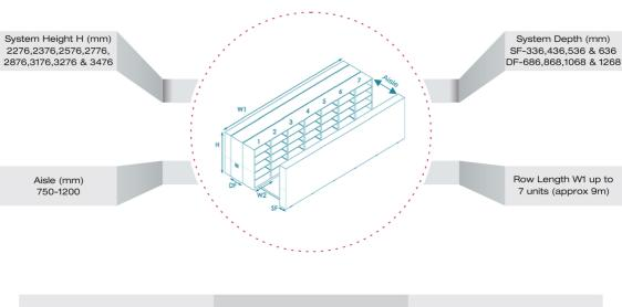
Shelf Panel (mm) Width W2-1300/body Depth-300, 400,500& 600 Usable Height (mm) 2111,2211,2411,2611, 2711,3011,3111 & 3311
