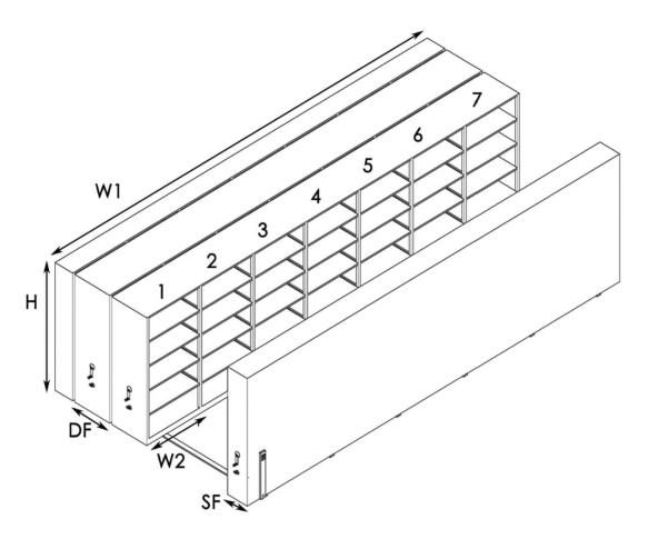
Unit Height, H - 1976, 2376, 2776 Unit Width, W2 - 1300 Number of Units - Upto 7 Overall Width, W1 - 9300 (for 7 units) All Levels are fixed
