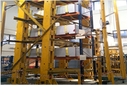
Tested seismic racking
